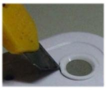
The retaining ring incorporates a cut-out section on the edge to allow prying of the ring out with a sharp knife to allow filter replacement if required.
