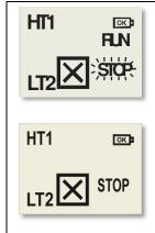
To stop the Indicator, press and hold the START/STOP button for 5 seconds
